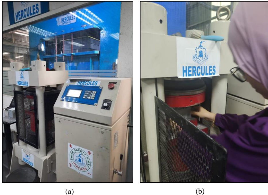
Figure 5. (a) Testing Cube Machine, (b) Placement of the cube in the testing machine
