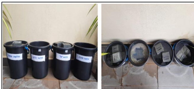
Figure 4. Water curing process (7 & 28 days)
