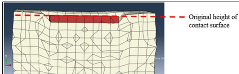
(b) Deformed shape of control with 1mm thick CFRP wrapping.
