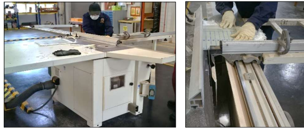
Figure 4. Specimen cutting process using Tenoning and Squaring Machine
