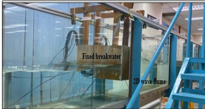
Figure 2. Fixed breakwater position in a 2D wave flume
