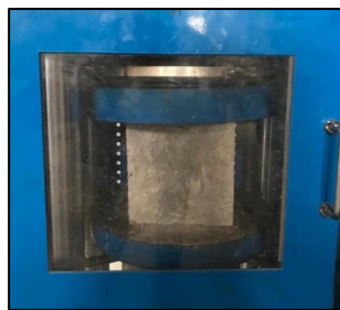
Figure 3. Compression test setup (BS EN 12390-3:2019, 2019)
