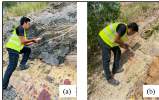
Figure 4. Schmidt Rebound hammer test conducted on (a) mudstone and (b) sandstone layer
