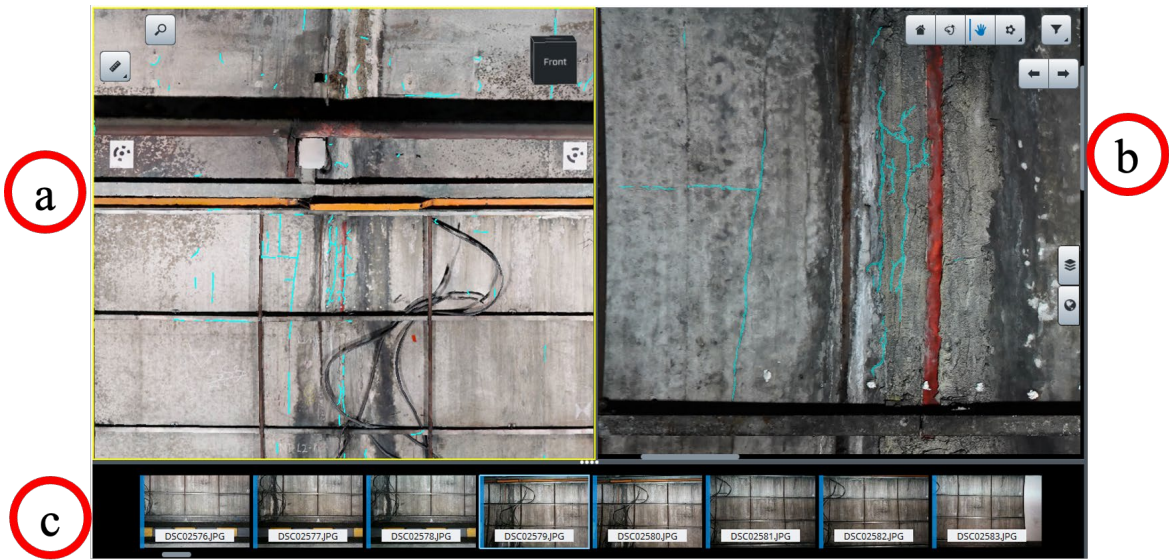
Figure 3. Crack detection visualisation in the iTwin interface. (a) Reconstructed 3D model of the tunnel wall showing segmented cracks overlaid in cyan, (b) Corresponding 2D oriented photograph with segmentation overlay, and (c) Image thumbnails used for model reconstruction.
