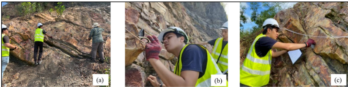
Figure 3. Scanline survey: (a) Establishing scanline of 15 meters (b) Measuring dip angle and dip direction of the discontinuity (c) Determination of JRC using Comb Profiler
