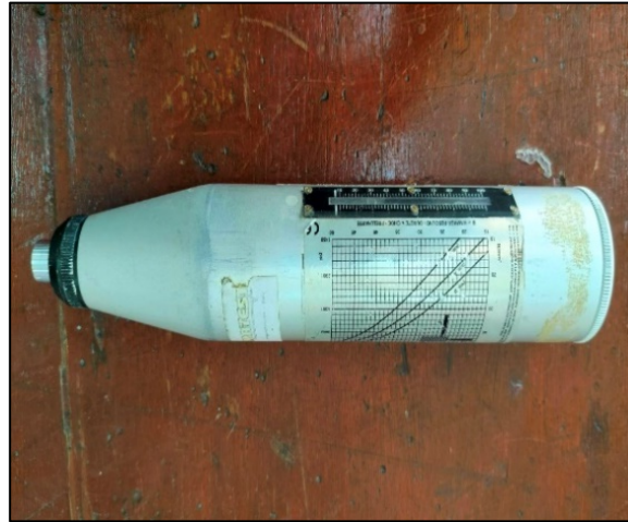
Figure 2.5 Rebound hammer apparatus.
